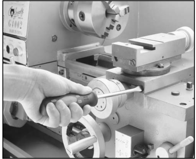
Figure 25. Adjusting the cross-slide gib.
